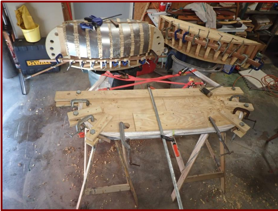
Bending the stem/keelson using the poly tube method.
