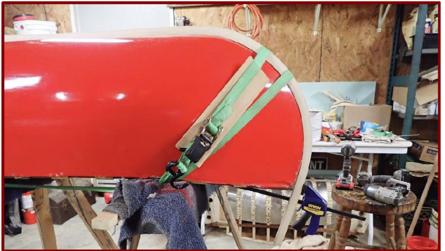
Attaching the outside stems.
