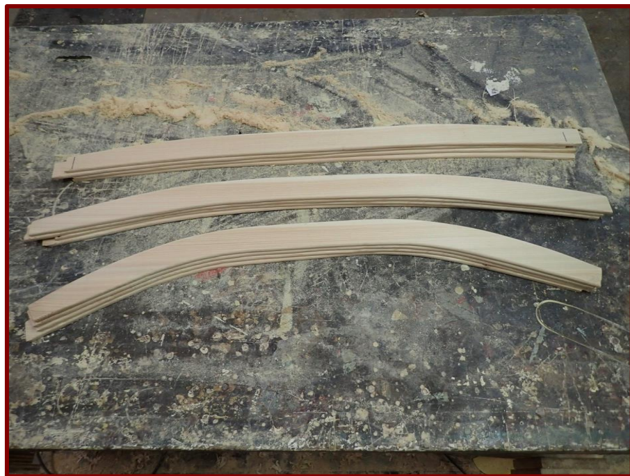
Curved ribs. Note the grain runout on the curviest ones. Not good.
