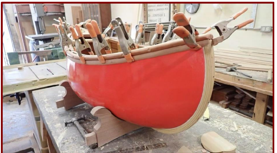
Attaching the cherry outwales and shaping the rocker cradle.
