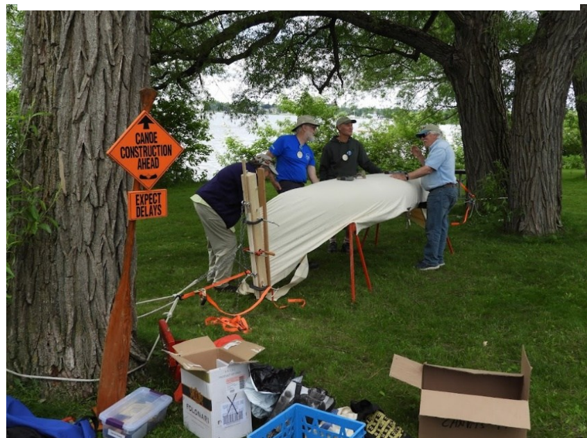
Photo 7: WCHA members recanvassing a 14' Huron canoe. Photo: Alex Guthro
