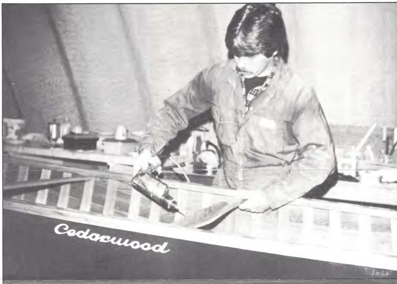
Steven Jones mounts a yoke thwart in a nearly finished sixteen-foot Prospector.
