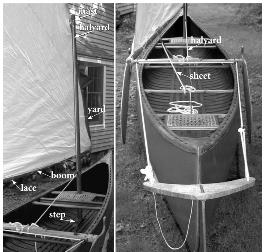
Rig details showing the boom, the yard, the step and the mast and the lines—lace, halyard and sheet.
