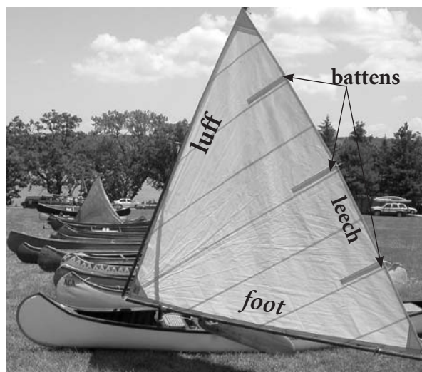
The sides of a sail—the luff, the leech and the foot—and the battens.
