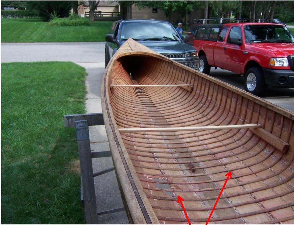
Ragged tapered edge on inside both garboards...
